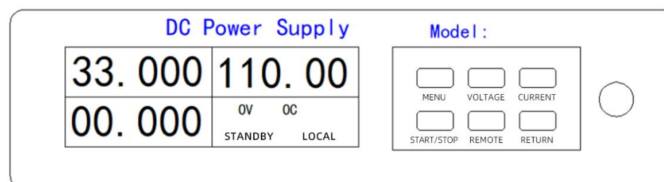
Figure 5-4 Overvoltage And Overcurrent Settings Interface
